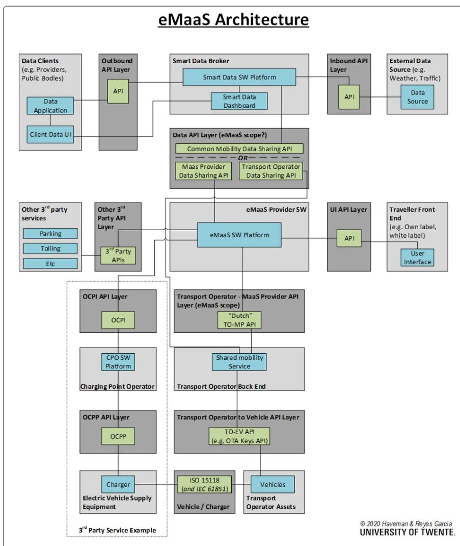
Figure 11 – eMaaS Software Architecture with a focus on roles & interfaces<sup>18</sup> (adapted)
